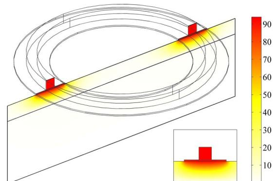
FIG. 9. (Color online)  $\Delta T$  map in a slice of the 3D structure and detail showing almost constant  $\Delta T$  in polymer loading.
