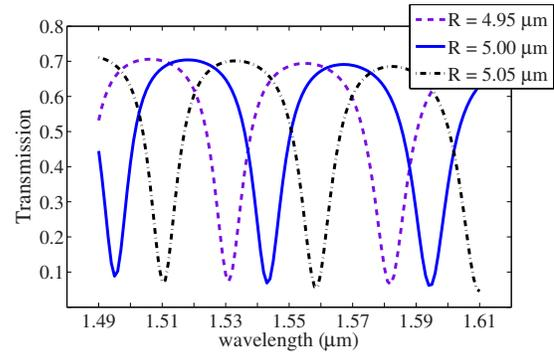
FIG. 5. (Color online) Transmission vs wavelength for slight variations in the ring radius. A variation of  $50 \text{ nm}$  results in a shift of up to  $15 \text{ nm}$ . The gap is fixed at  $0.25 \mu\text{m}$ .
