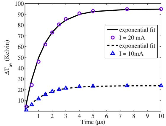
FIG. 11. (Color online) Temporal evolution of the average in the loading temperature increase for driving currents of 10 and 20 mA. Fitted curves indicate a time constant of  $1.35 \mu\text{s}$ .
