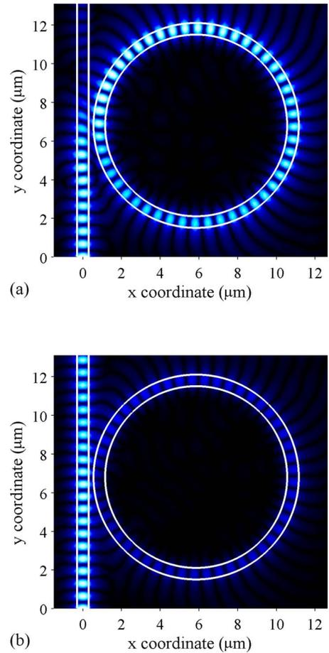
FIG. 3. (Color online) Absolute value of real part of  $E_z$  ( $|\text{Re}[E_z]|$ ) (a) at a transmission minimum ( $\lambda=1.594 \mu\text{m}$ ) and (b) at a transmission maximum ( $\lambda=1.568 \mu\text{m}$ ). The  $E_z$  component is plotted at an  $xy$  plane located 10 nm above the metal surface. The ring radius is 5  $\mu\text{m}$  and the gap is equal to 0.25  $\mu\text{m}$ .
