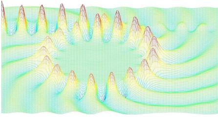
FIG. 7. (Color online) Augmented bend losses in the case of  $R=3.5 \mu\text{m}$  ( $g=0.1 \mu\text{m}$ ). The real part of  $E_z$  is depicted at an  $xy$  plane 10 nm above the metal surface. The operating wavelength is  $1.586 \mu\text{m}$  corresponding to a transmission minimum.
