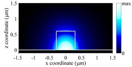
FIG. 2. (Color online)  $TM_{00}$  guided mode of the DLSPP waveguide, which consists of a  $600 \times 600 \text{ nm}^2$  polymer ridge deposited on a 70-nm-thick gold film. The  $E_z$  component is depicted for an operating wavelength of  $1.55 \mu\text{m}$ . The field enhancement near the metal-dielectric interface is evident.
