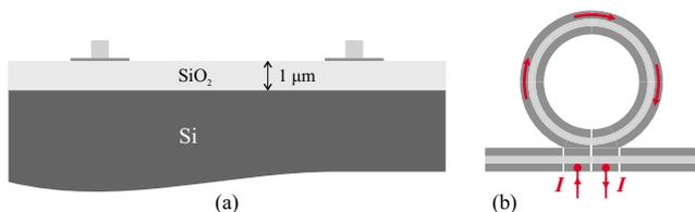
FIG. 8. (Color online) (a) Cross section of the computational domain considered in the thermal modeling simulations. (b) Possible practical layout of electrode placement resulting in an azimuthal current covering the entire circumference of the ring.
