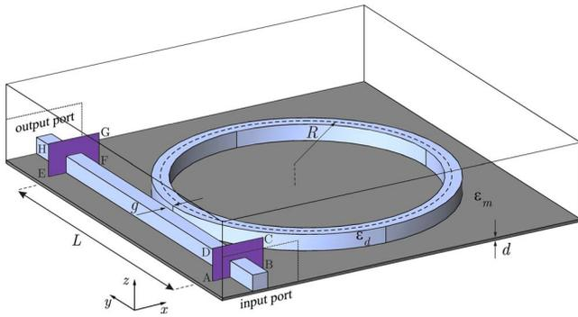
FIG. 1. (Color online) Schematic of a DLSPP-based microring resonator filter. The cross section at which the output power is calculated is marked as EFGH and is separated by a distance  $L$  from plane ABCD at which the reference power is calculated in the absence of the ring.
