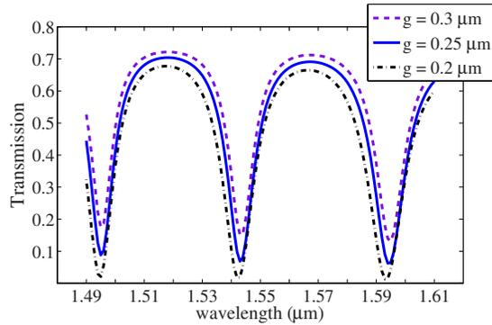
FIG. 4. (Color online) Transmission vs wavelength for different values of the gap separating the bus waveguide from the ring. The ring radius is equal to  $5 \mu\text{m}$ . The respective extinction ratios in the three cases are 7.35, 10.5, and 17 dB.
