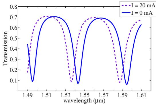
FIG. 10. (Color online) Transmission vs wavelength for the thermally tuned filter ( $R=5 \mu\text{m}$  and  $g=0.25 \mu\text{m}$ ). For a driving current of 20 mA, an 8 nm shift in the transmission minima is observed.
