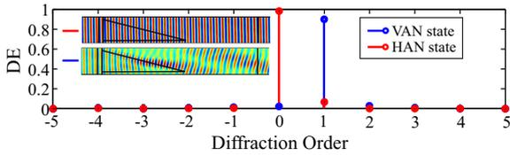
Fig. 3. Efficiencies of the diffraction modes for  $m = -5, \dots, 5$  for the proposed ZBD beam steerer. Inset shows the profile of the  $E_x$  component for both states. All geometrical parameters are as in Fig. 2.
