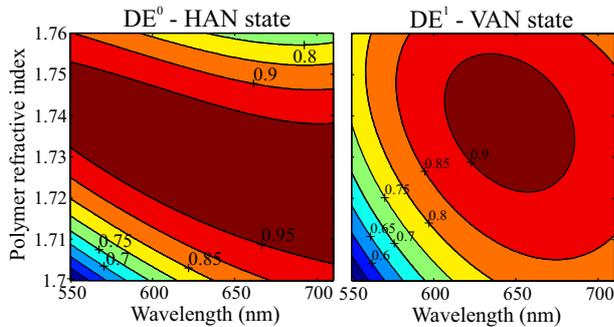
Fig. 5. Dependence of the diffraction efficiency for the  $m = 0$  and  $m = 1$  modes of the HAN and VAN states, respectively, on the operation wavelength and the polymer index.
