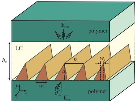
Fig. 1. Schematic layout and parameter definition of the proposed zenithal bistable liquid-crystal blazed grating.
