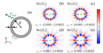
**Fig. 2.** (a) Nonlinear ring resonator considered in this work.  $R = 0.79 \ \mu\text{m}$  and  $w = 200 \ \text{nm}$  throughout. (b-e) Field plots ( $E_z$ -components) of resonance modes (of azimuthal order *m*) with gradually increasing radiation damping, owing to the decrease in Re{ $\varepsilon_r$ } that weakens field confinement. The permittivity values are 12.093, 10.093, 8.093, 6.093 for the four cases respectively and the imaginary part equals -0.0022 throughout.
