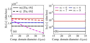
**Fig. 3.** Nonlinear feedback parameter calculations,  $\tilde{\kappa}_{ucj}$  and  $\kappa_{cj}$ , versus computational domain diameter *d* for the four resonant modes in Fig. 2. (a) Real part (Re{ $\kappa$ }): as radiation damping increases, the conjugated formulation breaks down but the unconjugated one remains unaffected. (b) Imaginary part (Im{ $\kappa$ }): Linewidth modifications can only be predicted by the unconjugated framework.
